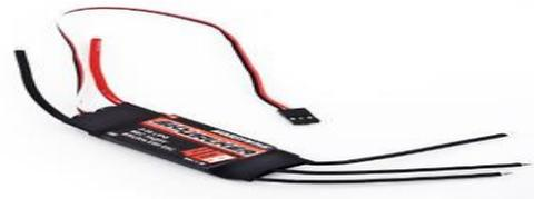
Fig. 4. Electronic speed controller.
