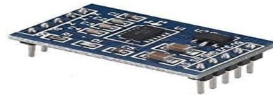
Fig. 5. Accelerometer sensor.
