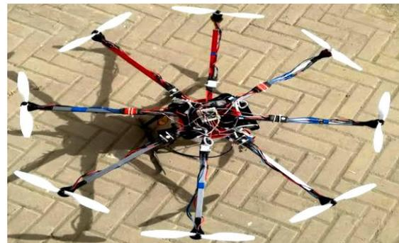
Fig. 8. Octocopter fabricated structure.
