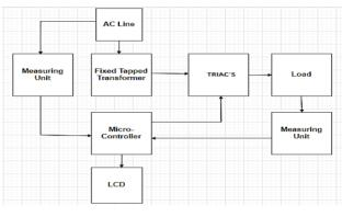
Fig. 1. Block diagram of TRIAC based voltage Stabilizer.
