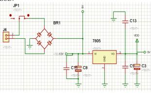
Fig. 5. Power supply circuit for AVR.
