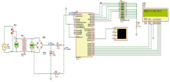
Fig. 6. Power stage circuit for AVR.
