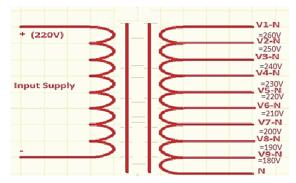
Fig. 3. Multi tapped transformer for AVR.
