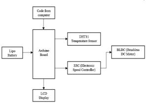
Fig. 7. Block diagram to control the motor speed.
