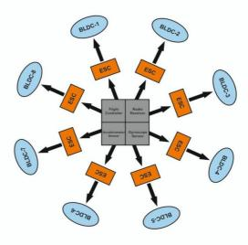
Fig. 1. The physical structure of the system.
