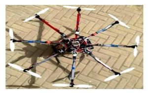
Fig. 8. Octocopter fabricated structure.
