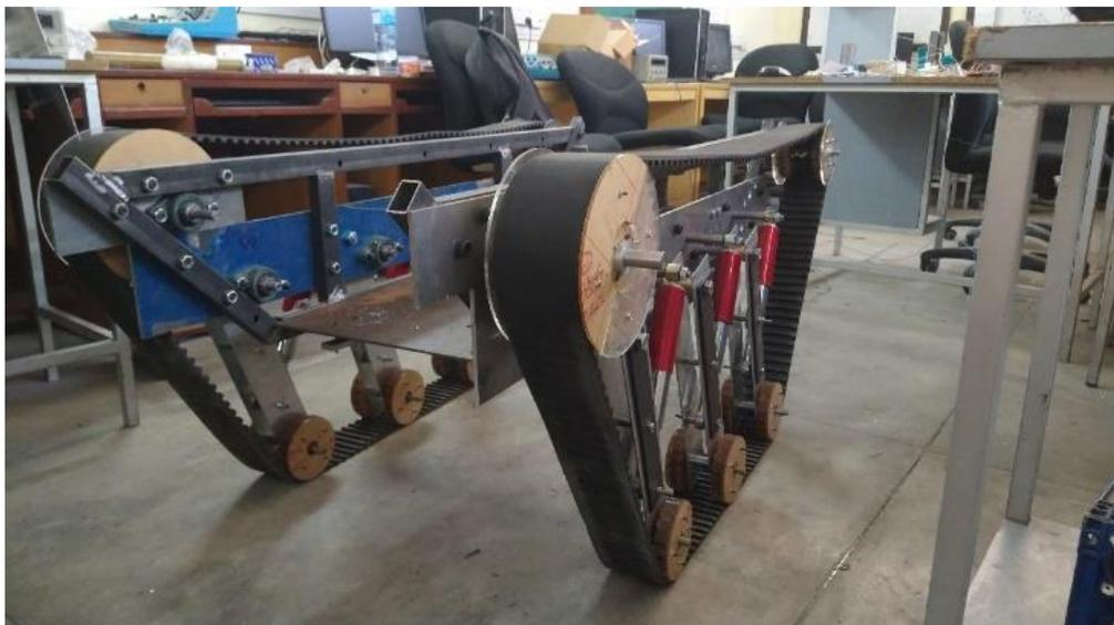
**Figure 17** / Fully Assembled Chassis and Track Mechanism
