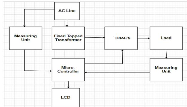
Fig. 1. Block diagram of TRIAC based voltage Stabilizer.
