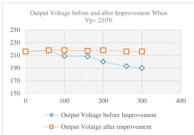
Fig. 9. Comparison of output voltages before and after improvement.
