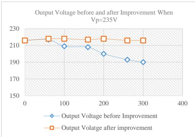
Fig. 7. Comparison of output voltages before and after improvement.
