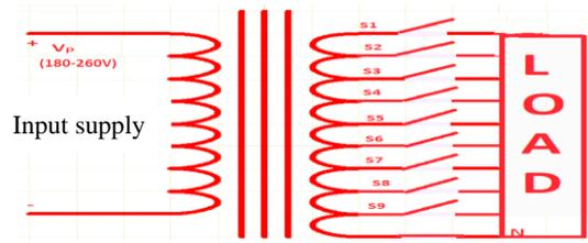
Fig. 4. Transformer connected with loads through switches.
