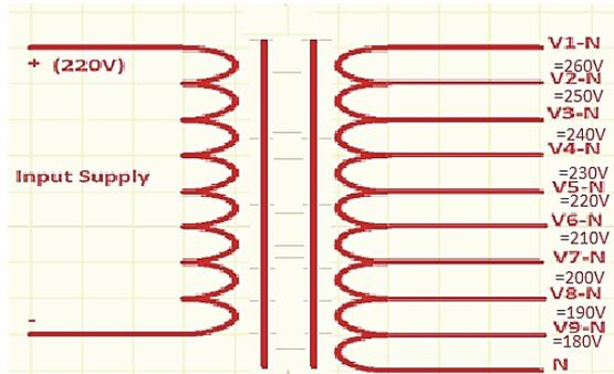
Fig. 3. Multi tapped transformer for AVR.
