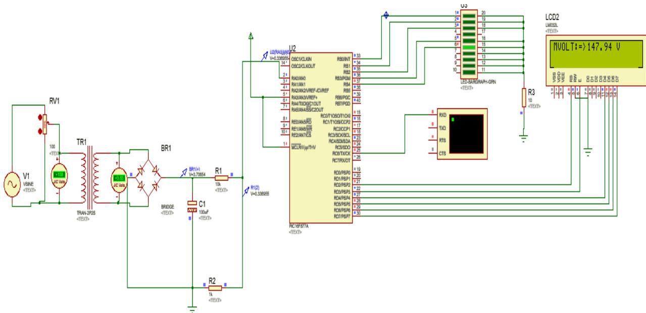
Fig. 6. Power stage circuit for AVR.
