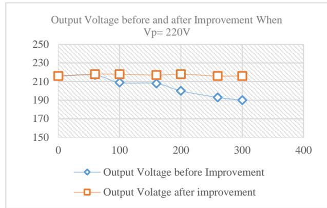
Fig. 8. Comparison of output voltages before and after improvement.
