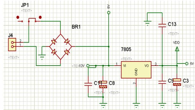
Fig. 5. Power supply circuit for AVR.
