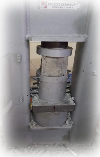
Fig. 12. Testing of WSA Modified Concrete Cube.
