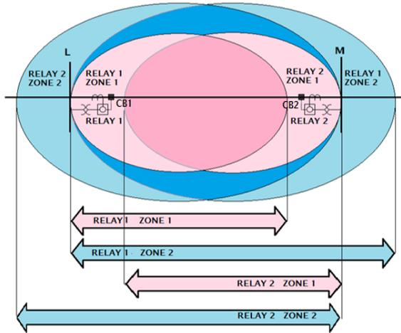
Fig. 3. Distance protection scheme for line LM.
