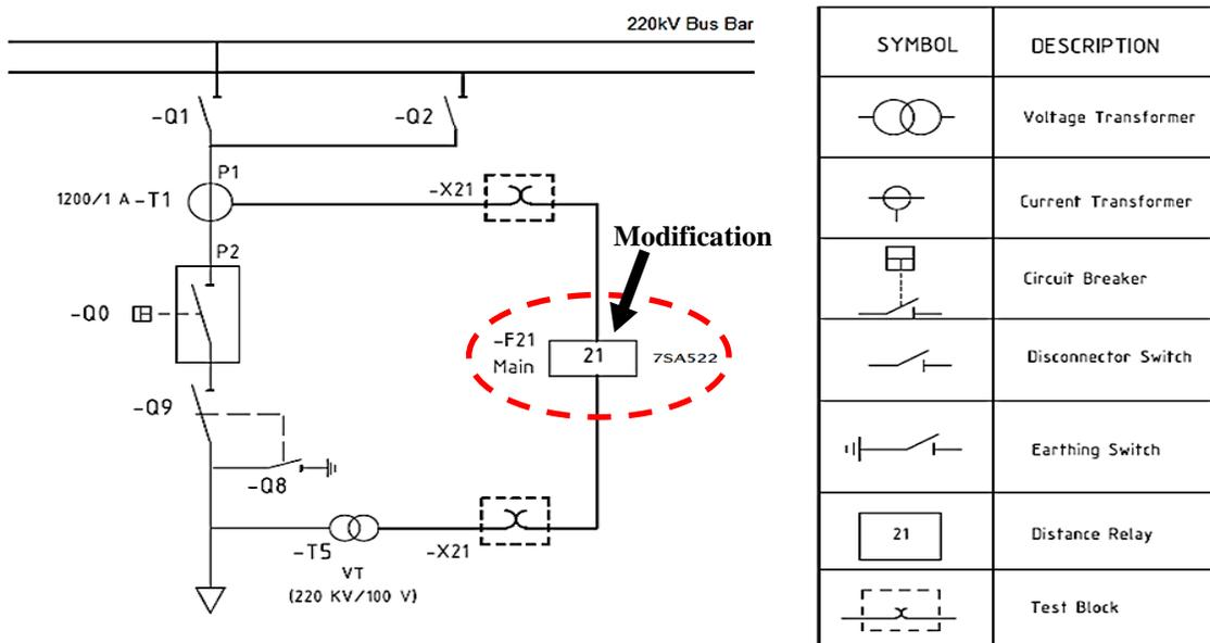
Fig. 12. Circuit Diagram of Modified Scheme.
