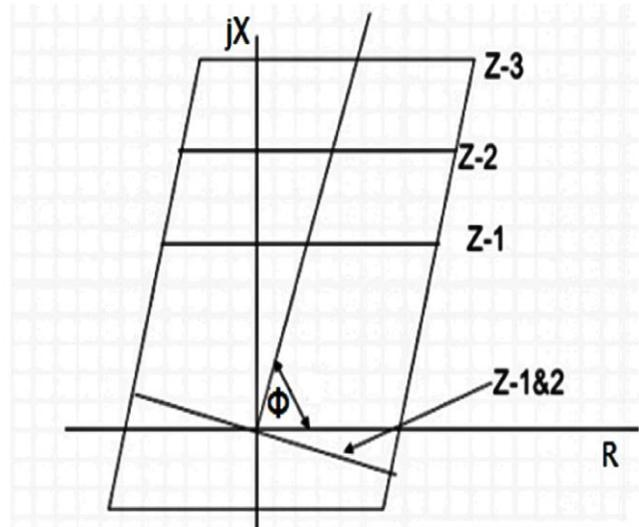
Fig. 2. Quadrilateral MHO characteristic.
