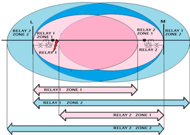
Fig. 6. Fault Occurring on Line LM near Bus L.
