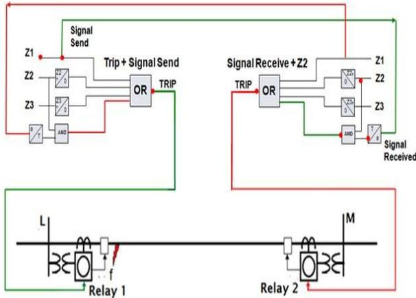
Fig. 8. Logic Diagram of PUTT Scheme.
