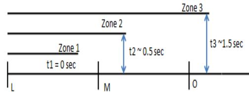
Fig. 1. Typical 3-zone Distance Protection.
