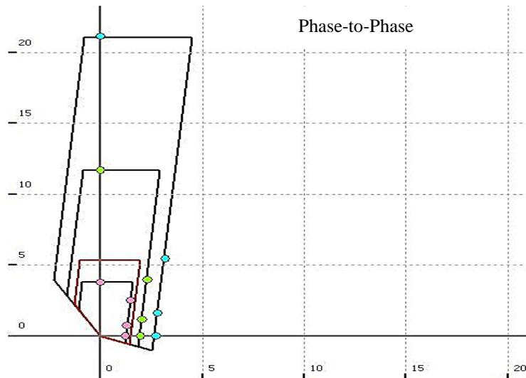
Fig. 18 L1-L2 fault injections in various zones of the protected line.
