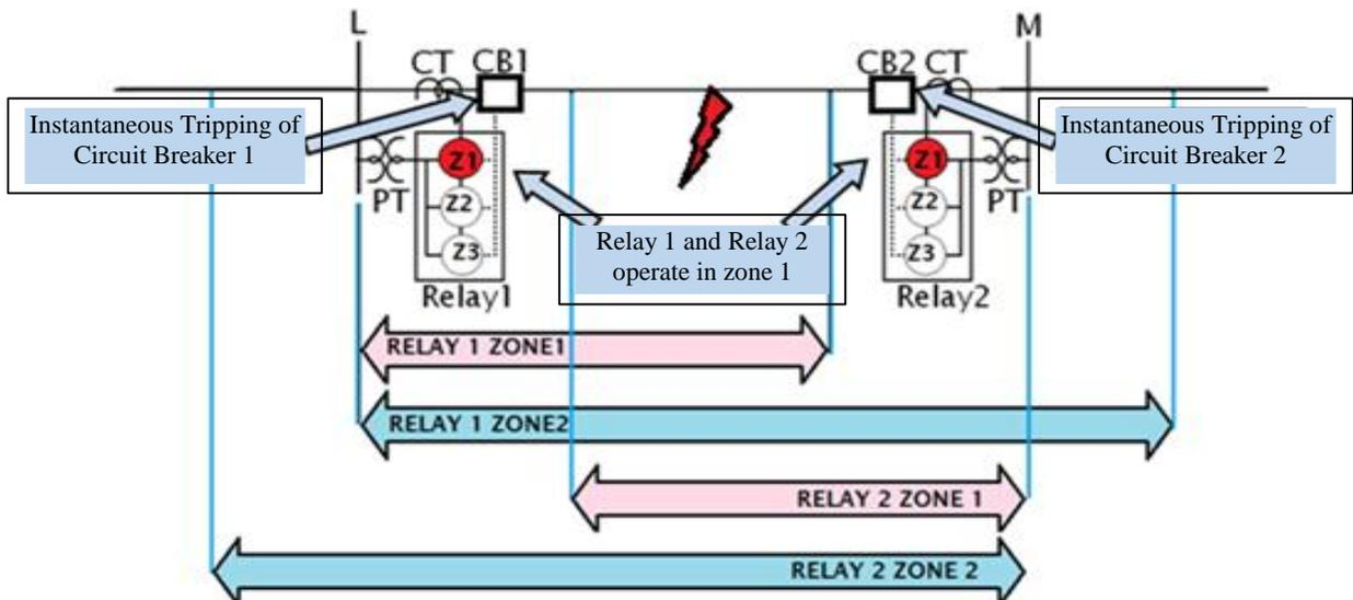
Fig. 5. Distance Relay coordination for a fault at middle of line LM.
