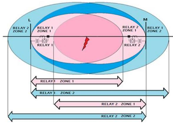
Fig. 4. Fault occurrence at middle of the Protected Line.
