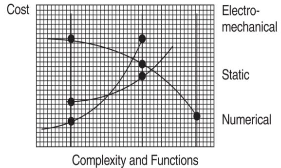
Fig. 9. Relay Comparison
