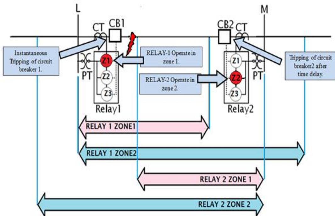
Fig. 7. Distance Relay Coordination for Fault on Line LM near Bus L.
