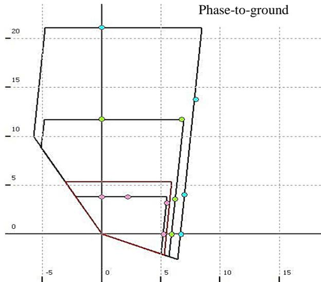
Fig. 17 L1-G fault injections in various zones of the protected line.
