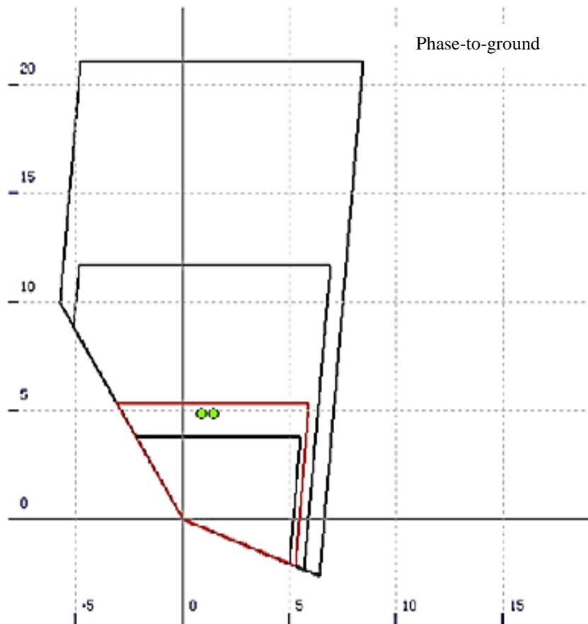
Fig. 20 L1-G fault injections in various zones of the protected line with tele-protection setting.
